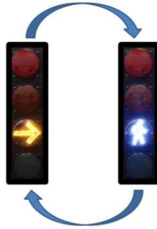
Figure 2-1 - Supplemental signal warning for right-turning motorists [55]
